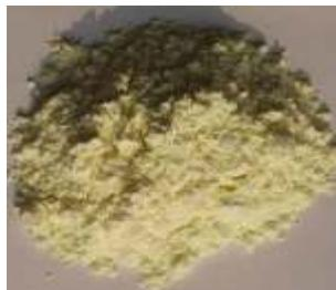
Endothermic and exothermic foaming agents. Specially modified for the rotational moulding process. Excellent results to add mechanical and insulating properties of products. Applications in multi layer tanks, transport boxes, rigid containers and insulated walls.
